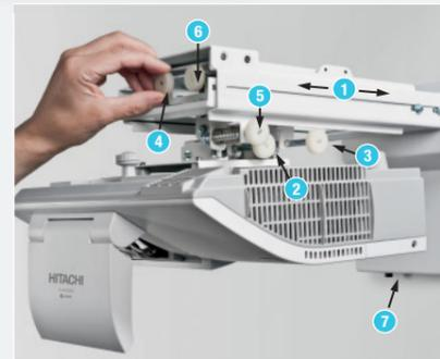
For fine adjustment all 6 axis can be individually corrected using the large dials located on the exceptionally versatile Hitachi mount. The diagrams opposite show how each dial can correct an image. In addition there is a fine vertical adjustment which can move the entire image up or down.
