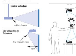
Ultra Short Throw – Using Hitachi's new unique high performance lens. We are able to dramatically reduce the throw distance, combined with the introduction of a high angle projection capability, the quiet ED-A101/ED-A111 projector can be sited only 42cm away for a 60" screen.
